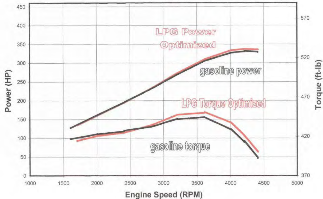
GM 8.1 Liter Engine Full Load Comparisons
