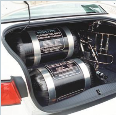
Fuel tanks in car trunk
