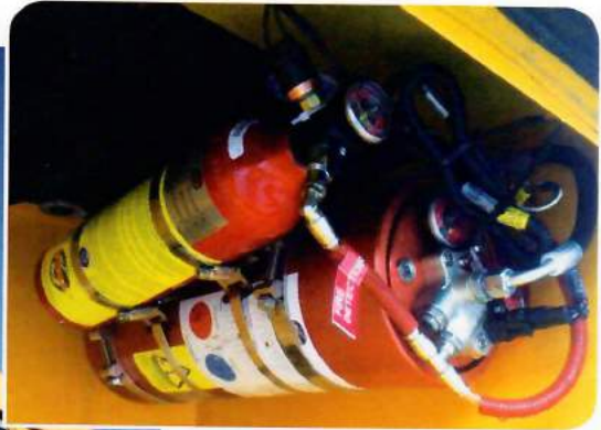
National Express, which includes Durham School Services, will add the Fogmaker fire suppression system (above) on its new school bus purchases.
