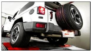
Thanks to the technologies available at the Holdim group, our chassis dynamometers have been provided with a hydraulic link supporting realistic road simulations in all the engine working conditions while testing cars/light vehicles, heavy duty trucks and buses, tractors and motorbikes.
