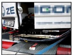
Portable Emission Measurement System, lightweight laboratory which purpose is to test and assess emissions on mobile sources during on-the-road tests or in dynamometer sessions. This service can be offered also on site by our specialized technicians.
