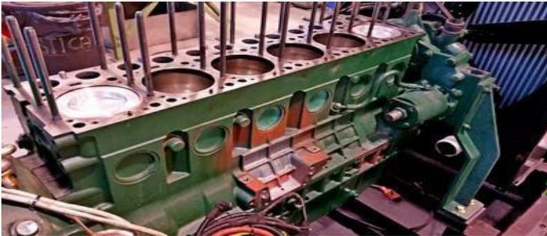
Conversion of Diesel engines to 100% Natural Gas spark ignited Otto cycle with phased ignition
